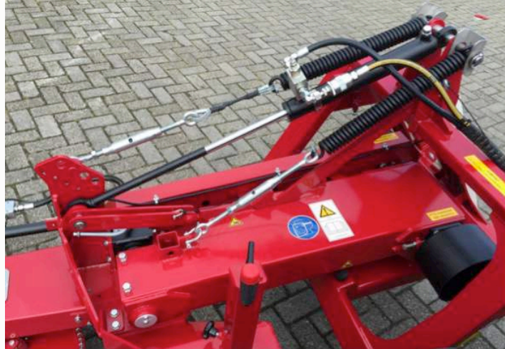
Parallelogram construction with relief springs
