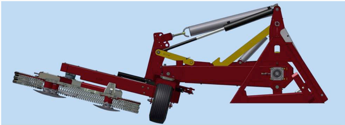
3D example of 5° lifting (N.B. support wheel is not applied!)
