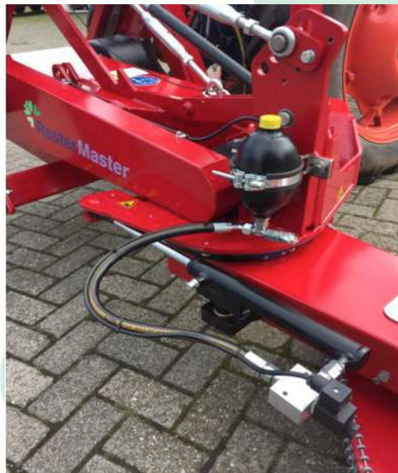
Hydraulic arm cylinder with accumulator
