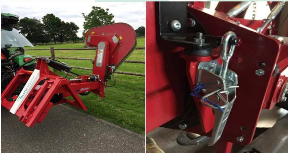
Transport position and locking of cutter arm
